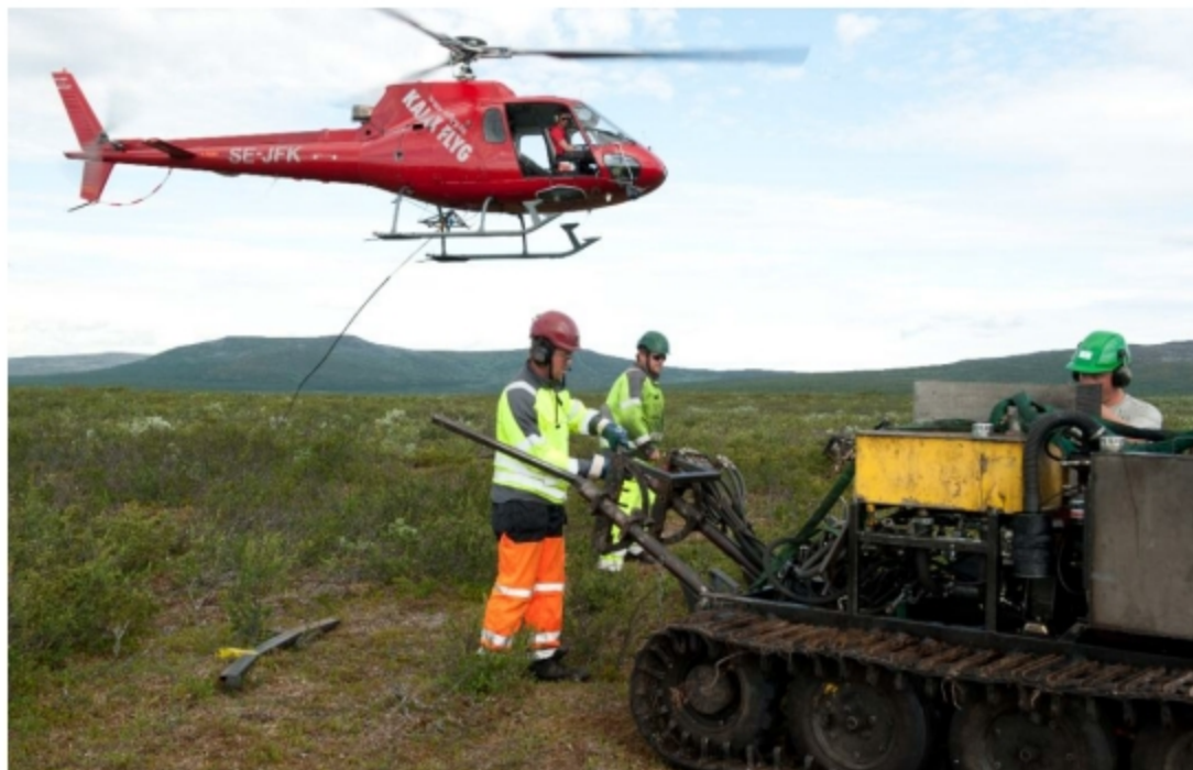
A drilling rig is transported to the prospecting area by helicopter to protect the environment
